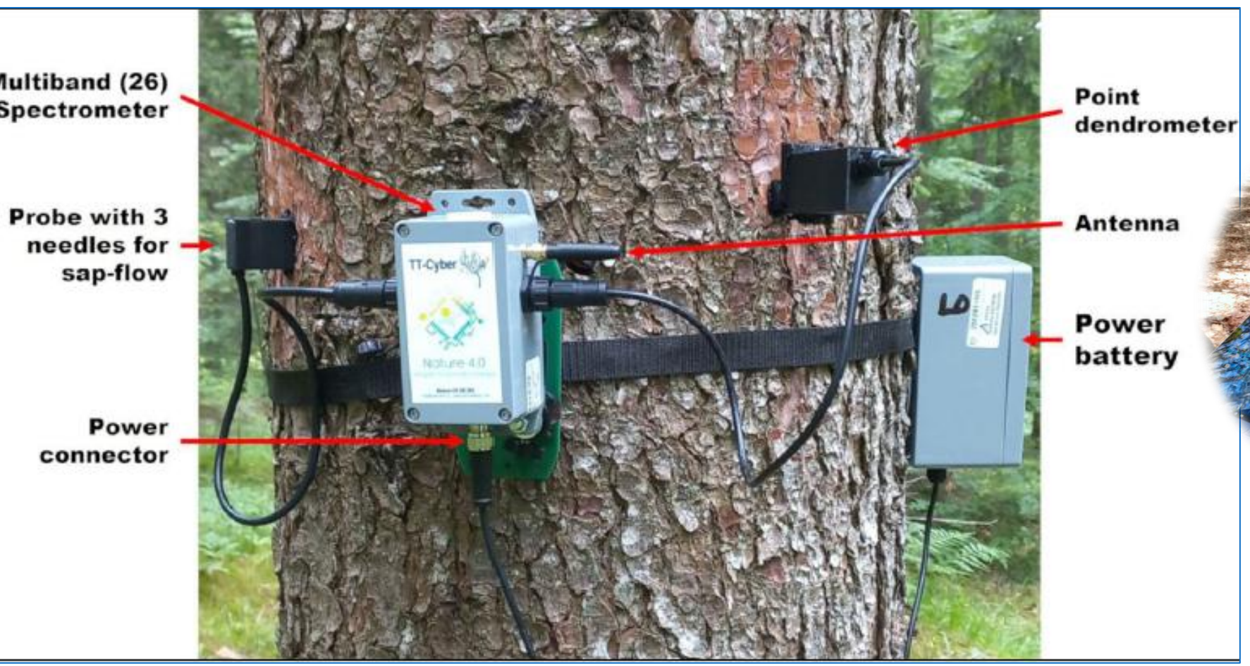
Figure 1. Tree Talker device to collect real-time tree data.
